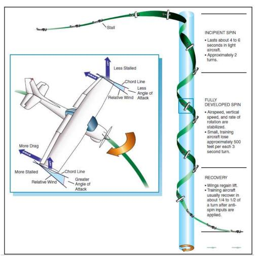
The first think you should take note of is a stall occurs first. In fact, you cannot spin an aircraft without first stalling it. The main characteristic of a fully developed spin is that one wing is more deeply stalled (creating more drag and less left) than the other wing. That is what a spin is, but not all aircraft will spin, should be spun, or if spun may not recover. Here is a video of a Cessna 150 doing a spin. <u>http://www.youtube.com/watch?v=h2rm7n9Vz3c&feature=related</u>
