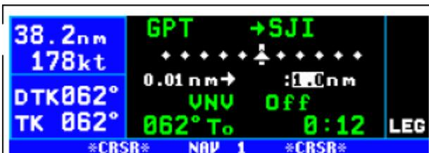
Press the **CRSR** button to highlight the full scale sensitivity number. Use the inner knob to select 1.0. Turn the **CRSR** off by pressing it again.
